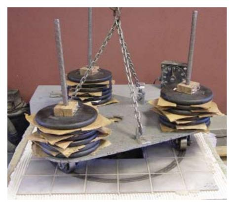
Above: The assembly pictured above is on cycle number 12. Once the cart has completed the 450 revolutions required by cycle 12, the sample will undergo a visual examination to determine whether or not cycle 13 will commence.
